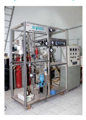
High Temperature single tube Catalytic fixed-bed reactors are the most important type of reactor for the synthesis of basic chemicals and intermediates. In these reators, the reaction takes place in the form of a heterogeneously catalyzed gas reaction on the surface of catalysts. In addition to the synthesis of valuable chemicals, fixed-bed reactors have been increasingly used in recent years to treat harmful and toxic substances.
